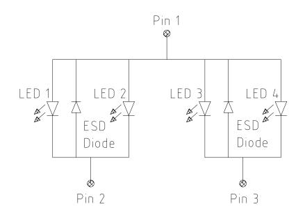
1: anode 2: cathode LED 1 and 2 3: cathode LED 3 and 4
